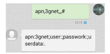
After the APN is set, please resend command of test# to check if GPRS is OK. If still NO, please double confirm with your network provider.
